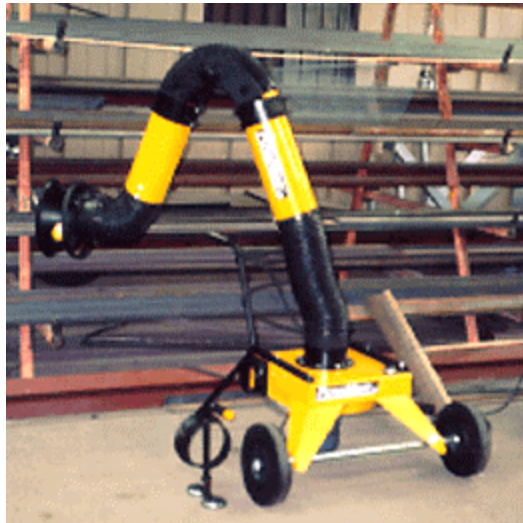
Figure 2: Local Exhaust Ventilation Unit 1 (MEF model)
