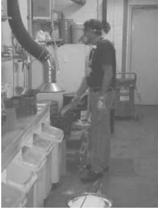
Weighing Cr(VI) pigment for colored glass production (Photo courtesy of the National Institute for Occupational Safety and Health (NIOSH)).
