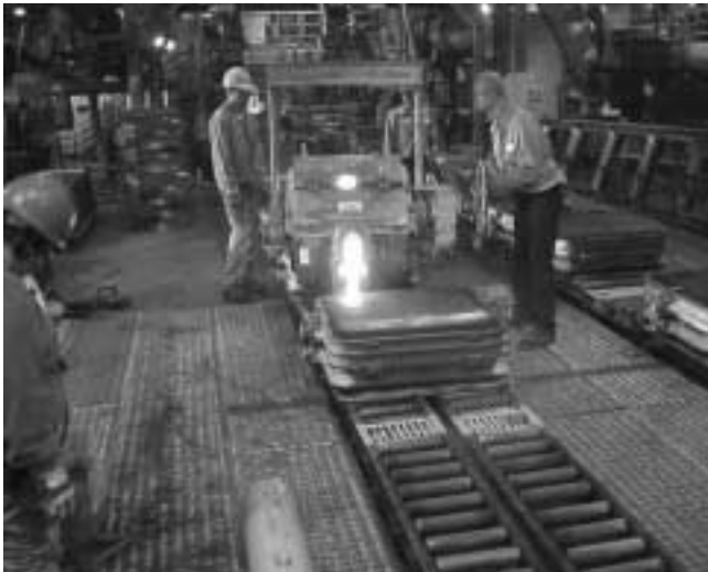
Filling molds in a foundry (Photo courtesy of the National Institute for Occupational Safety and Health (NIOSH)).
